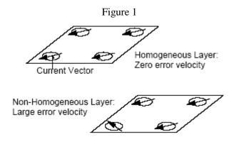
Error velocity requires that there are 4 beams being used to create an earth coordinate transformation. If a beam has been disabled (to avoid risers) or if a beam has gone bad the error velocity will have a value of -32768. To QA/QC the error velocity the first step should be to review the value of error velocity if it equals -32768 then skip this QA/QC setup and move to the next QA/QC step.
