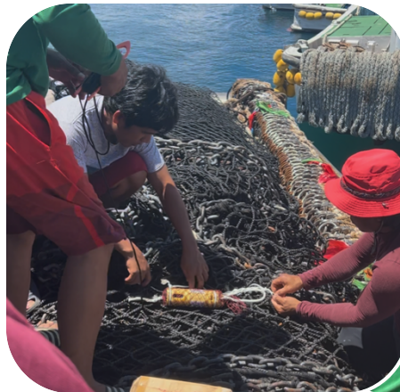
Figure 10. Fitting of the Moana sensor on a purse seine net using tough jacket #1 in a net bag, ~50cm above the lead line.
