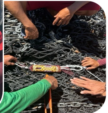
Figure 10. Fitting of the Moana sensor on a purse seine net using tough jacket #1 in a net bag, ~50cm above the lead line.
