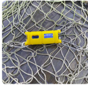
Figure 9. Moana sensor in tough jacket #3 directly attached to a net or woven in.
