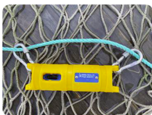
Figure 6. Alternate attachment for trawl, directly to net using a lead rope.
