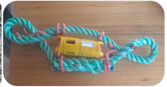
Figure 9. Moana sensor in tough jacket #3 directly attached to a net or woven in.
