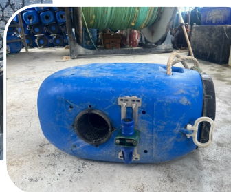
Figure 13. Moana sensors fitted to pots and traps using mounting plate and clamps designed for pots and traps, or sturdy cable ties for attachment to wooden pots.
