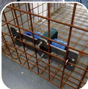
Figure 13. Moana sensors fitted to pots and traps using mounting plate and clamps designed for pots and traps, or sturdy cable ties for attachment to wooden pots.
