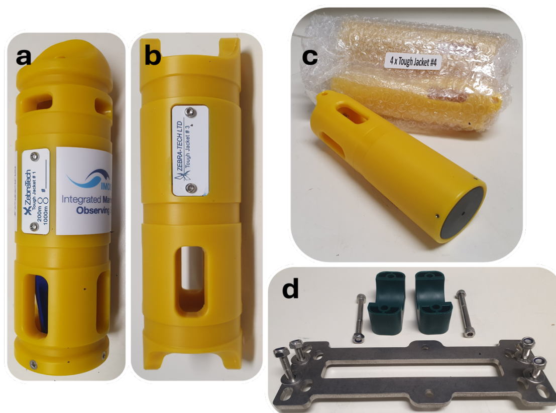
Figure 4 Attachments and protective housings for the Moana TD200 and Moana TD1000. (a) Tough Jacket #1 for purse seining applications; (b) Tough Jacket #3, the most versatile option suitable for various gear types; (c) Tough Jacket #4 designed for longlining; (d) Attachment option for use with pots and traps.
