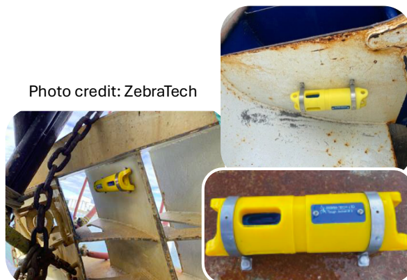
Figure 5. Moana sensor attached to trawl door using tough jacket #3 and brackets.
