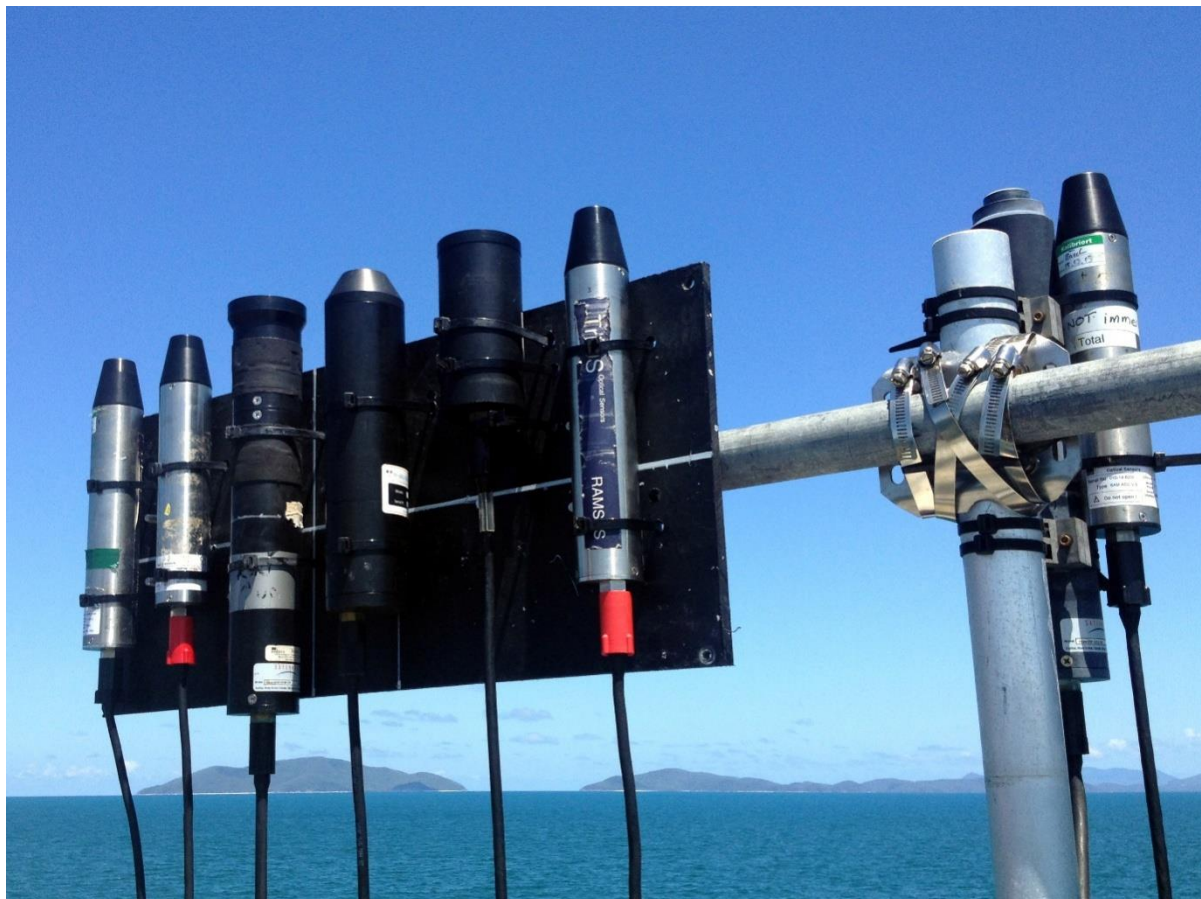
Figure 13: Irradiance Radiometers: from right to left, RAMSES 5039, RAMSES 8035, HyperOCR 346, USSIMO 0002, MS8 Prototype, RAMSES 506D, IMOS HyperOCR (not included in the RTT lab and field inter-comparison) and RAMSES 8375. The smallest instrument (5 th from the left) is a prototype multispectral sensor not included in this work.
