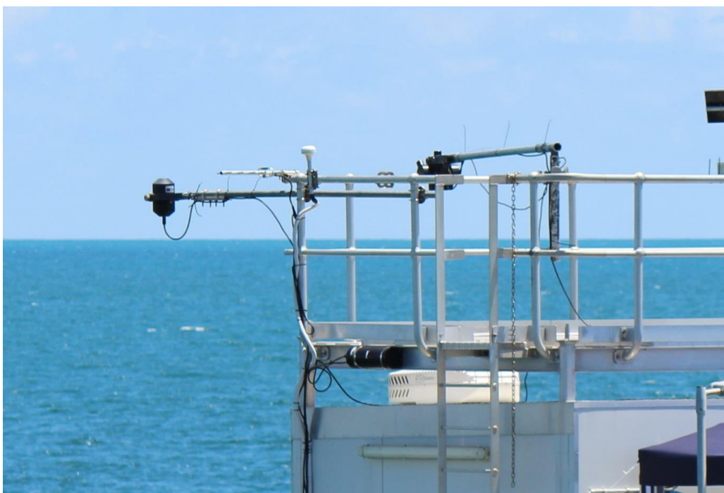
Figure 14: The boom-mounted DALEC spectroradiometers (IMOS DALEC on left, Curtin DALEC on right).
