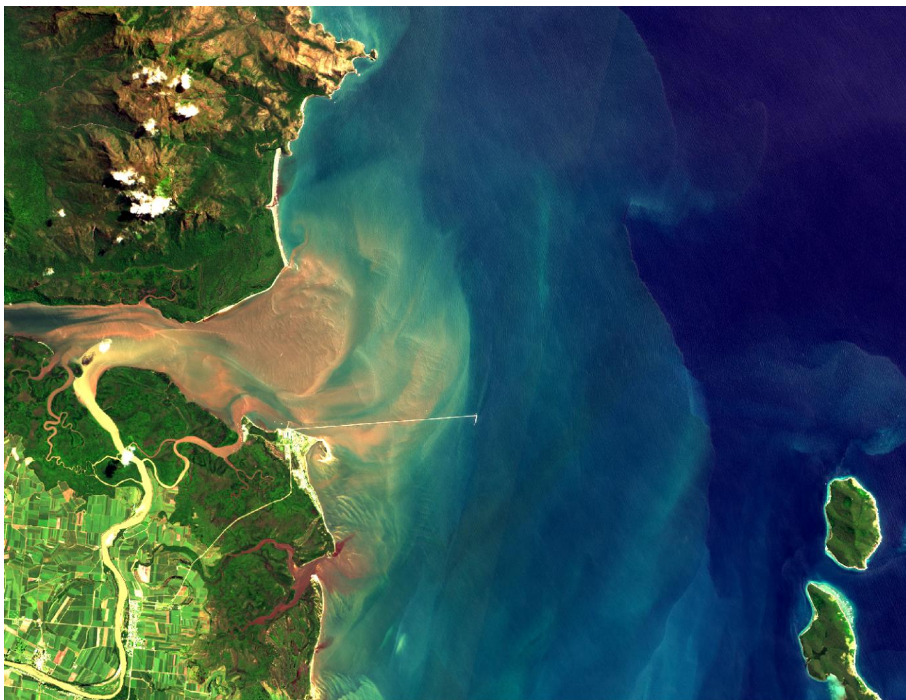
Sentinel2-MSI true colour image taken above the Lucinda Jetty Coastal Observatory (LJCO). The observatory is located at the end of a 6-km long jetty, which appears clearly as a white strip in the image. The spatial resolution of this image is 60m. © ESA, Copernicus Australia
