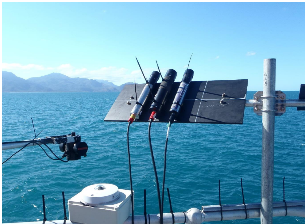
Figure 16: Radiometers attached to black panel in Sky Radiance Mode (Curtin DALEC in background on the left, where the L_t sensor head can be seen pointing to the ocean, 40^\circ from Nadir. The other side of the DALEC features the L_{sky} sensor which is pointing to the sky, 40^\circ from Zenith. Hemispherical web-camera (not used for radiometric measurements) can be seen in the foreground, mounted to railing.
