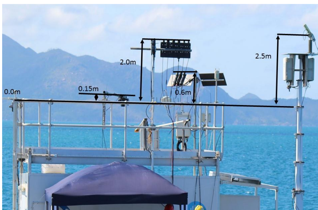
Figure 15: Approximate relative heights between cosine collectors (where applicable) and the handrail. Note - IMOS DALEC Irradiance cosine collector is level with the handrail.
