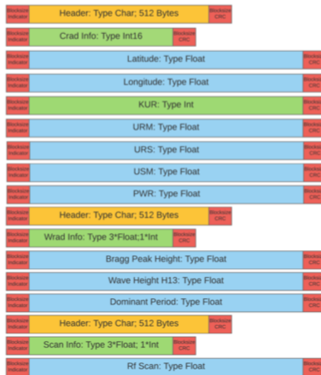
Figure 2. Structure of the merged binary file. The first block contains radial current information; single-radar wave information is stored in the second block. The third block contains a spectrum scan performed 2 minutes before the beginning of the acquisition cycle. WERA systems have the capabilities to dynamically adapt the operating frequency within the allocated frequency band, in attempt to decrease interference to normal operations. WERA HFRs managed by the IMOS Ocean Radar Facility however do not currently implement this feature.
